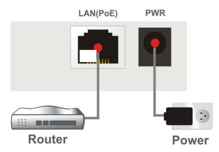
• Connect VigorAP to the PoE switch (via LAN port) with an Ethernet cable for getting the power from the switch directly. While connecting with a PoE switch, the power adapter is not necessary but optional.
