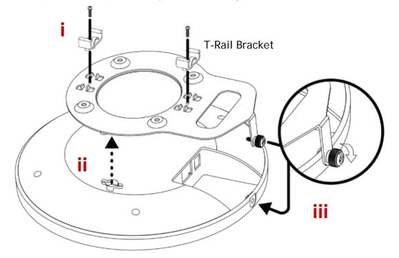
i. If a larger gap is required between the ceiling and the VigorAP, use the extension pieces to extend the height of the brackets.
